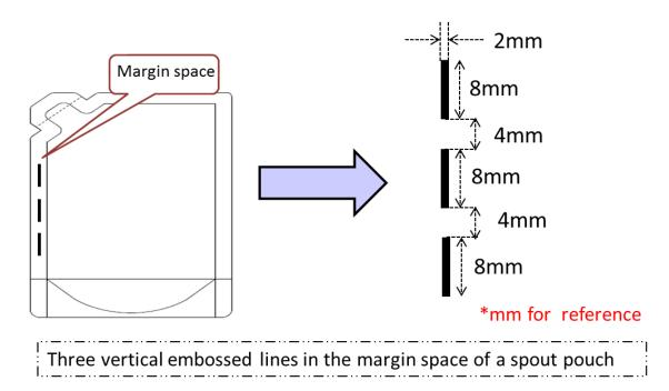
Note: When using cap at spout pouch, tactile identification symbol same as a general container may be alternatively displayed at the top of the cap.
