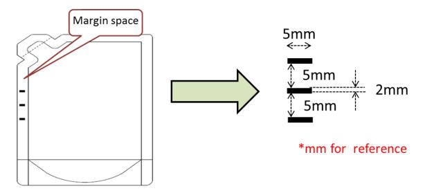
Three horizontal embossed lines in the margin space of a spout pouch
